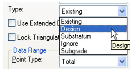
In order to later calculate volumes between two surfaces, one must be set to *Existing* and another to *Design*.
