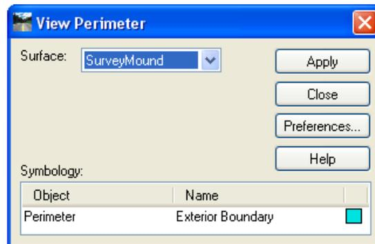
*The outer limit of the surface triangles is displayed in the design file*
